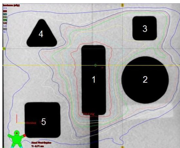
Figure 3. Dose distribution in the phantom with five cavities - isodose lines provided by planning system.
