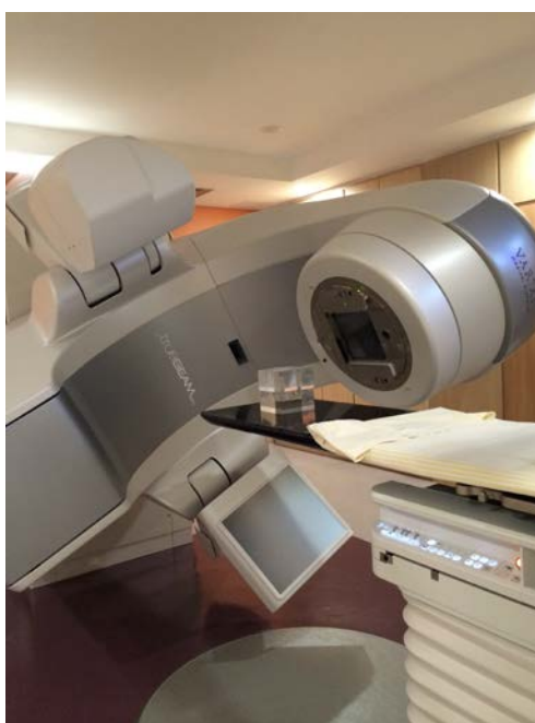
Figure 2. Set up of dosimeters irradiation using PMMA phantom with five cavities and linear accelerator Truebeam STx of Varian Medical Systems of HIAE.
