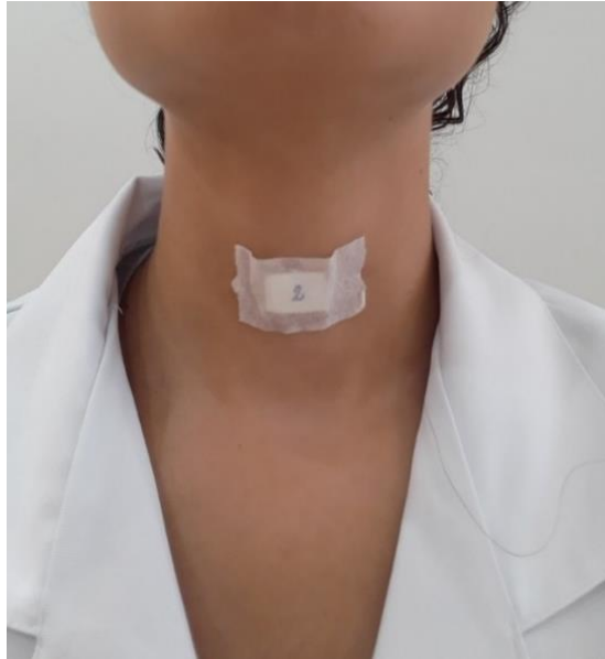
Figure 1: TLD package positioned near the thyroid (on the neck) of the volunteer.
