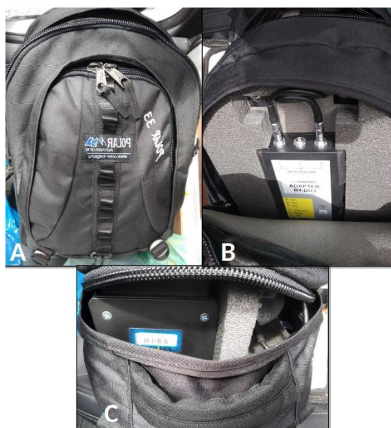
Figure 2: Spectrometry equipment. A) Case for transportation of equipment; B) Power and electronic modules; C) Gamma and neutron detectors.
