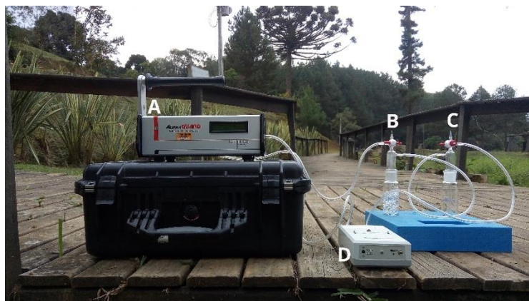
Figure 4: Schematic of the AquaKIT arrangement used for water measurements. A) AlphaGUARD detector; B) water sample; C) safety glass; D) Alpha Pump.
