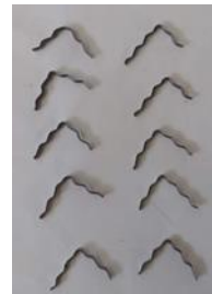
Figure 9: Steel fibers crimped after folding test.
