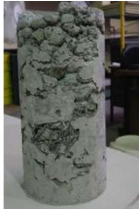
Figure 7: SFRC specimen with 1.5% vol of type A steel fibers with much voids.
