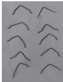
Figure 8: Steel fibers into hooked-end after folding test.
