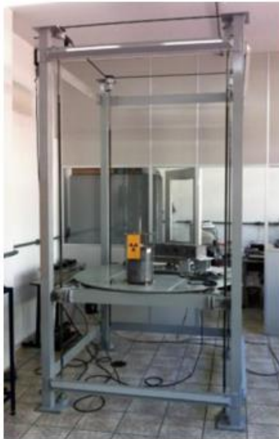
Figure 4: Third - generation industrial tomograph developed at IPEN / CNEN–SP.
