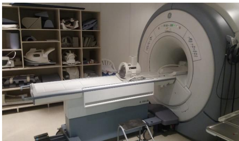
Figure 3: MRI equipment. Irradiated samples of the dosimeter gel were inserted into a head coil to obtain images.
