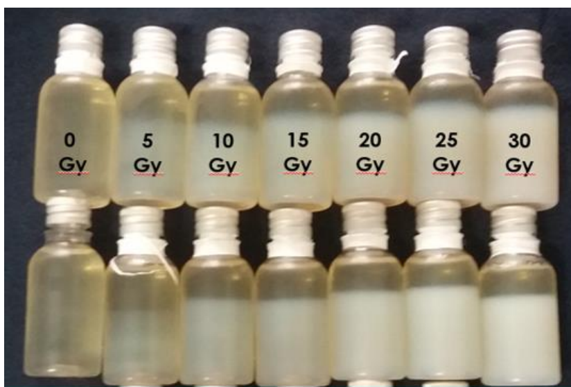
Figure 4: Samples of 30 g dosimeter gel irradiated with different dose values. From left to right in the image: 0, 5, 10, 15, 20, 25 and 30 Gy.
