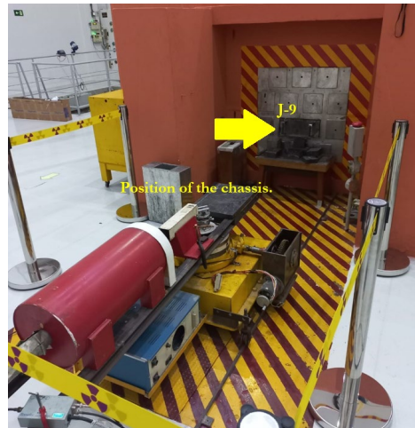
Figure 1: The position place of the J-9 channel and chassis in the Argonaut reactor.
