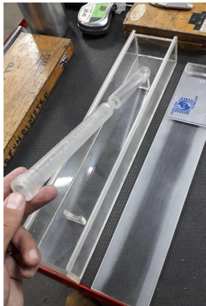
Figure 10: Adapter for ionization chamber type NE 2561.
