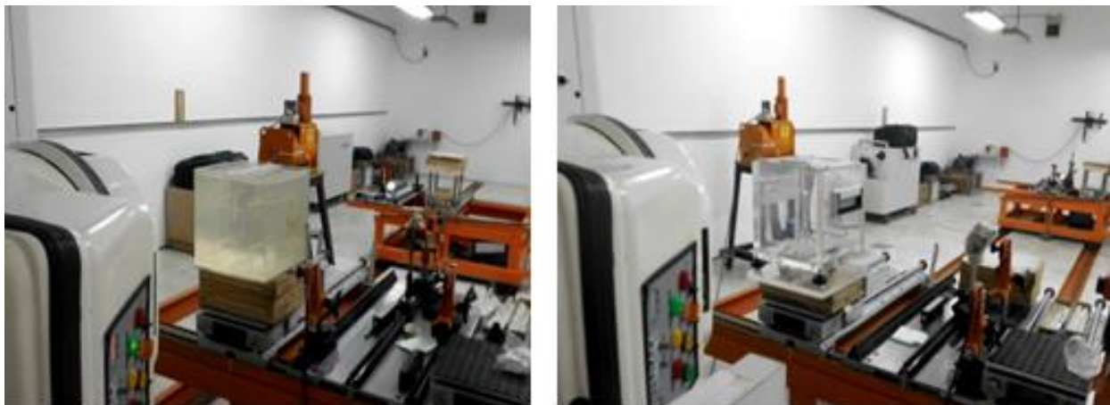
Figure 8: Positioning of the phantoms in the SSDL bunker in Venezuela.
