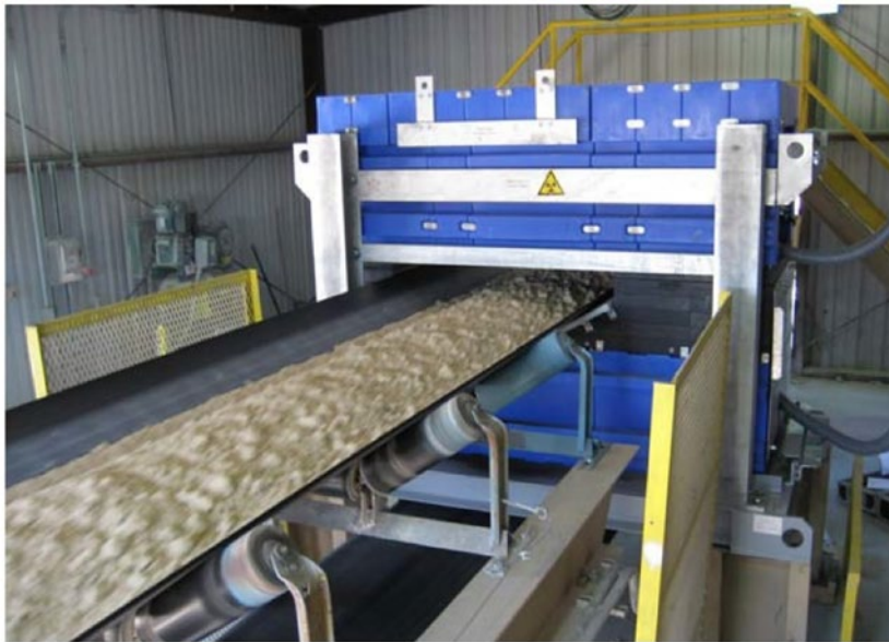
Figure 1: PGNAA analyzer situated directly on the conveyor belt.
