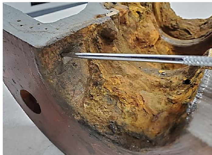
Figure 1: Example of a small pick being used on the inner surface of a valve to remove ductile material.
