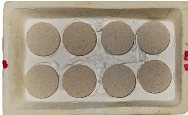
Figure 2: Pellets of glass and zeolite before sintering V2ZAC_Sr, V4ZAC_Sr, V6ZAC_Sr and V8ZAC_Sr from left to right.
