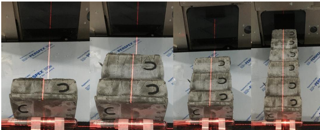
Figure 2: Top view of samples with different thicknesses being exposed to ionizing radiation in the linear electron accelerator. During the experiment, spacing between samples was not considered. The figure shows type “C” samples that refer to the T.BA.FA folder samples.
