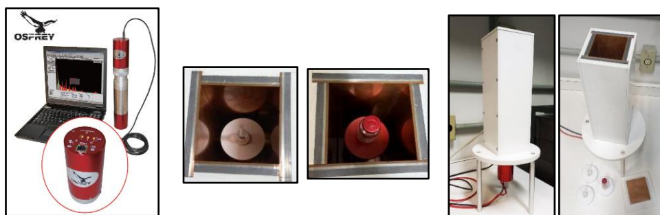
Figure 1: Arrangement of the gamma spectrometry system with NaI(Tl), containing the detector crystal, associated electronics, source holder, and lead shielding.
