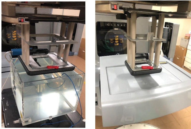
Figure 2: Illustration of the experimental setup used with diode and EPID.
