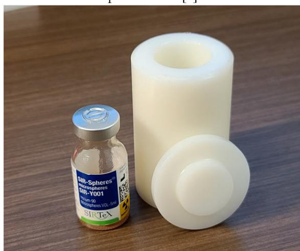
Figure 3. Photograph of custom high-density-polyethylene source holder and example SIR-Spheres patient vial [1].
