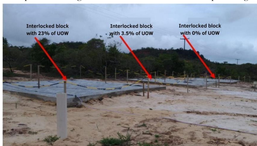
Figure 2: Outdoor experiment using cement blocks and preparation of the rainwater collecting system.
