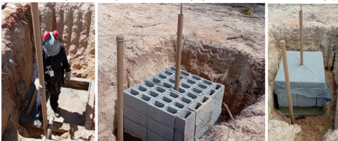
Figure 2: Outdoor experiment using cement blocks and preparation of the rainwater collecting system.
