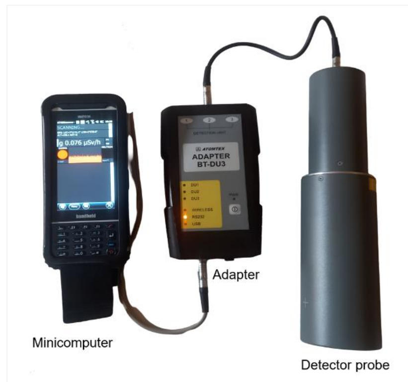
Figure 2: Photograph of the AT6101C(E) spectrometer used in this study to measure the ambient gamma dose equivalent rate.
