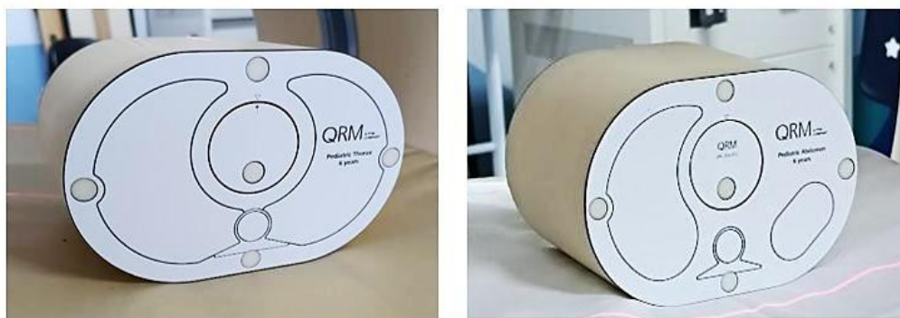
Figure 1: ATOM 007 phantom used for thoracic simulation and ATOM 007TE phantom used for abdominal simulation
