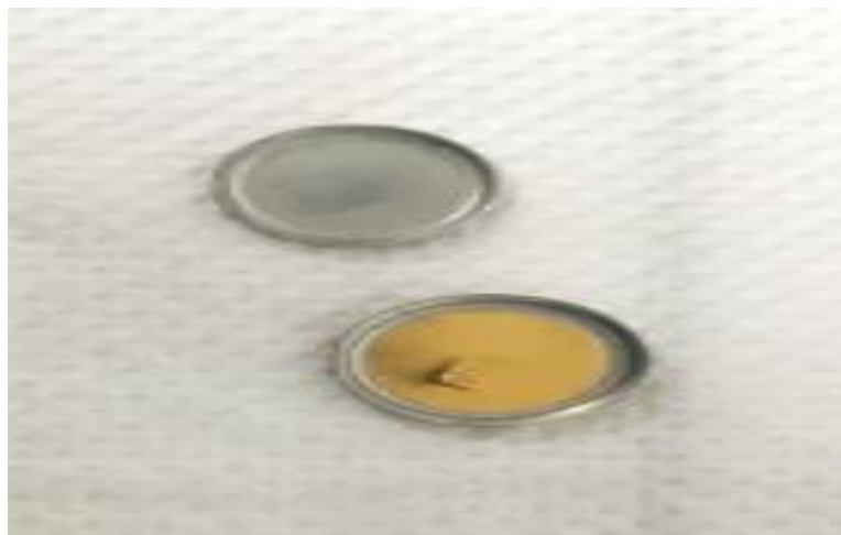
Figure 3: Gold foil with cadmium capsule belonging to LNMRI/IRD.
