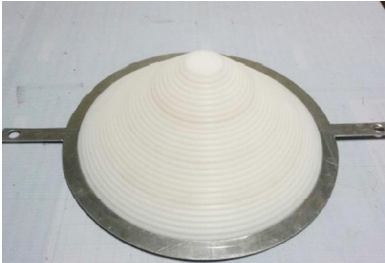
Figure 2: Filter with concentric conical polyethylene layers developed at LNMRI/IRD.
