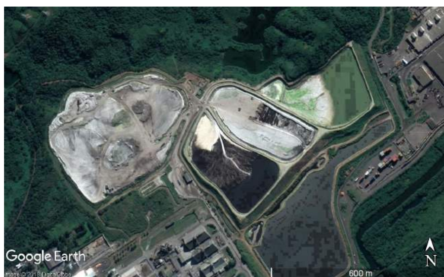
Figure 5: Phosphogypsum stack at Cubatão phosphate fertilizer complex (owned by Mosaic Fertilizantes) in 06/16/2017
