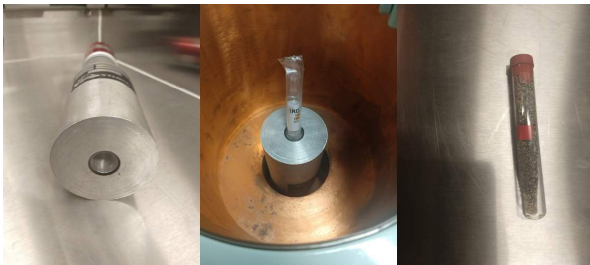
Figure 2: Counting geometry, calibration source and sample.
