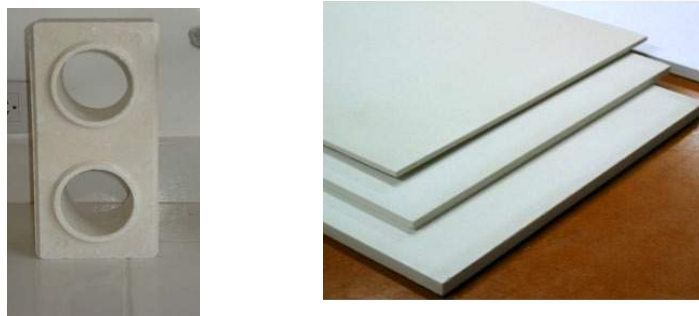
Figure 16: Bricks and plates made of phosphogypsum
