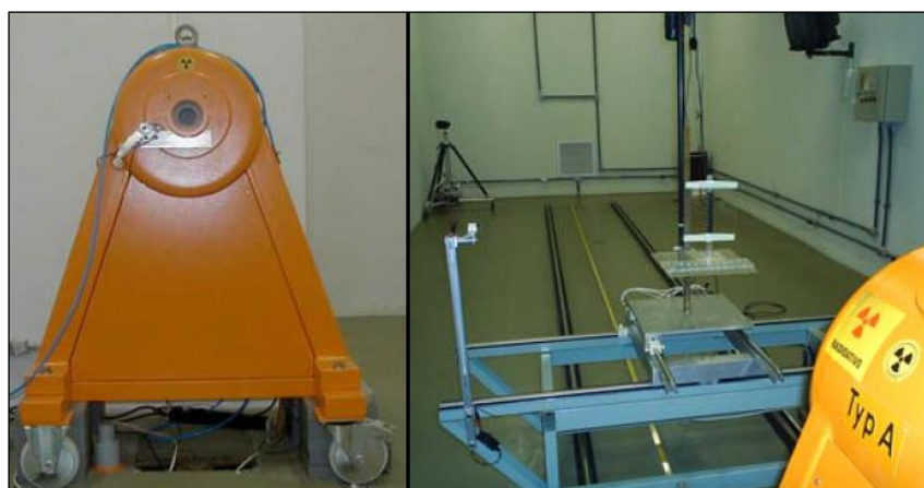
Figure 2: STS Model OB85 Irradiator.
