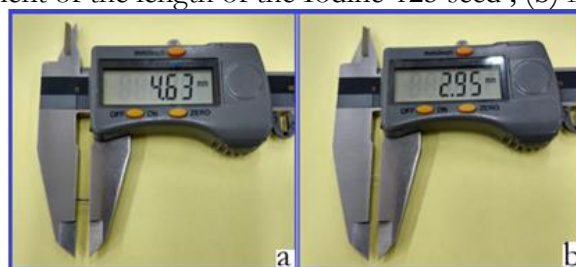
Figure 2. (a) Measurement of the length of the Iodine-125 seed ; (b) Measurement of the core.
