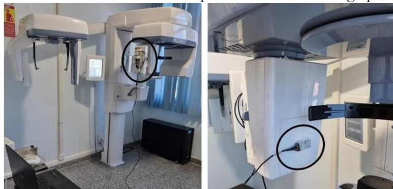
Figure 2: Detector Accu Gold AGMS-D positioned on the tomograph image receptor
