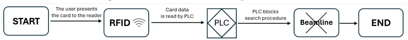
Figure 8: Data flow for PLC blocking forbidden cards
