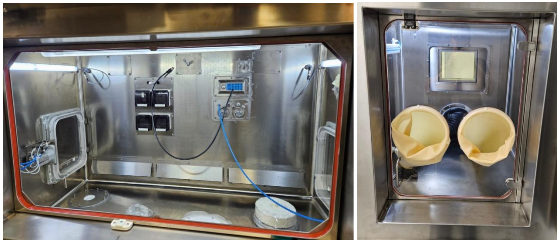
Figure 2: DC and RIC internal chambers with pneumatic gaskets.
