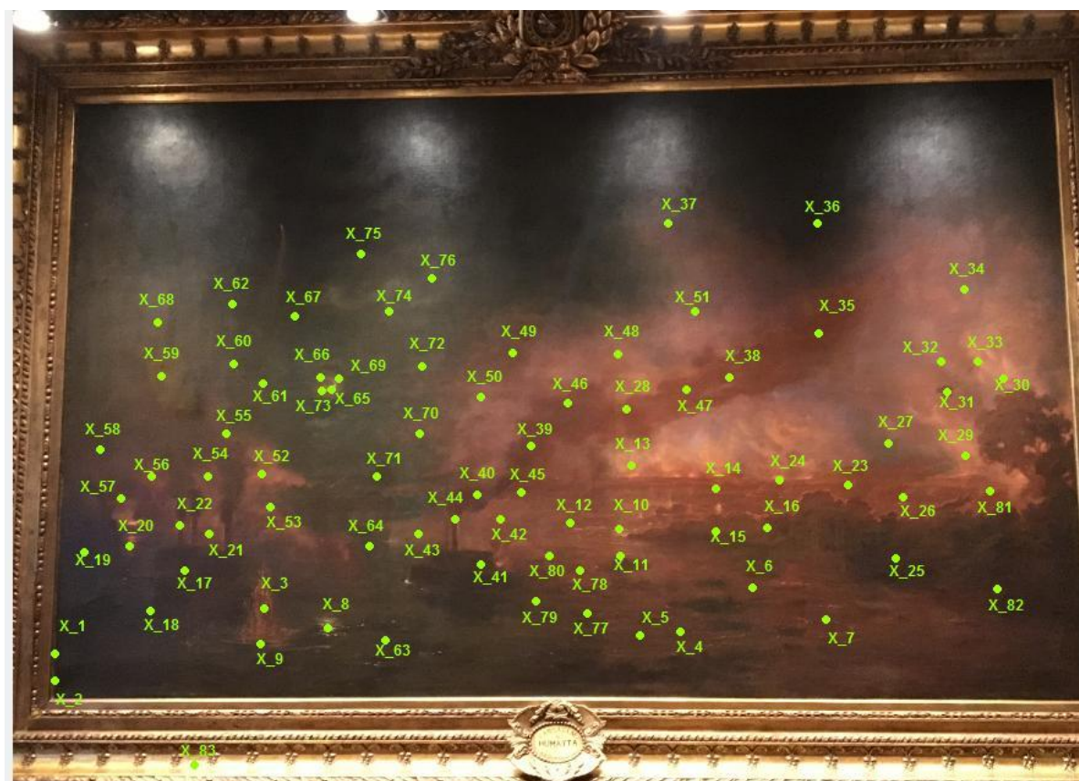
Figure 1: The canvas “ Passagem de Humaitá ”, with the points and where were registered, the spectra by XRF.
