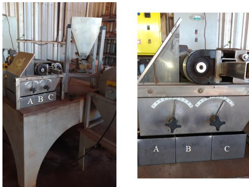
Figure 6: Magnetic separator used. In A is deposited the non-magnetic, in B the magnetic and in C the mixed.
