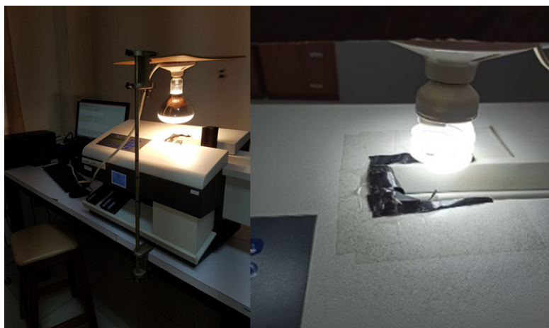
Figure 2: Photo of the measuring conditions using the two types of light bulbs (left side of figure 100 W light bulb and right side 20 W light bulb)
