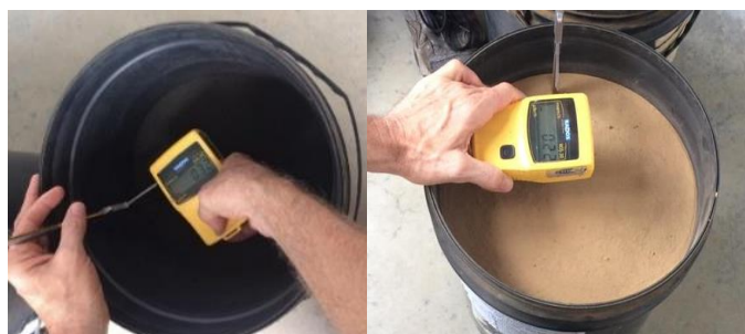
Figure 4 - Detection of surface activities and measurement of dose rate
