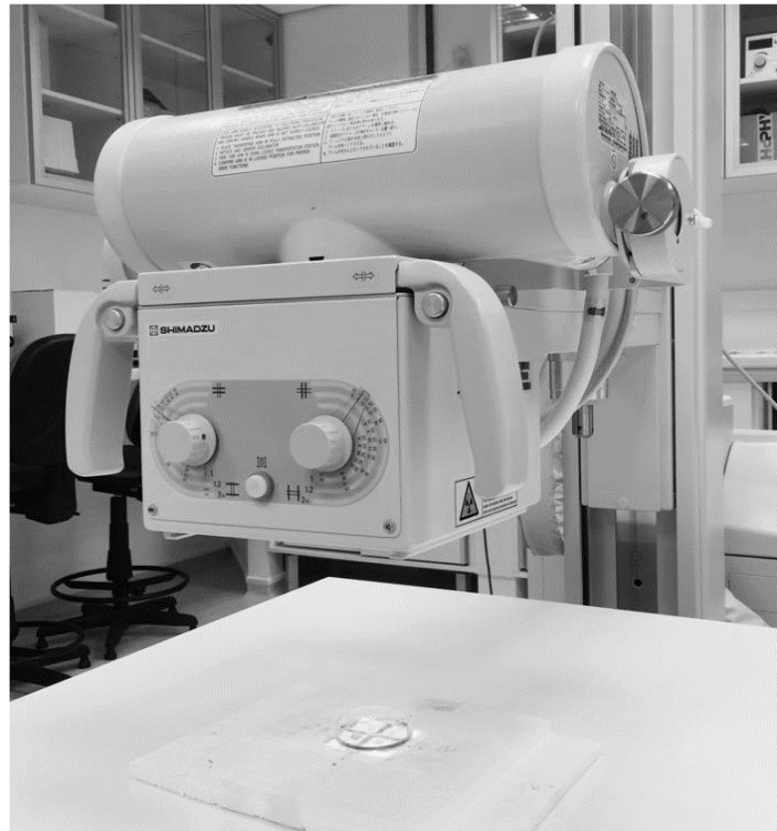
Figure 2: TLDs exposure scheme
