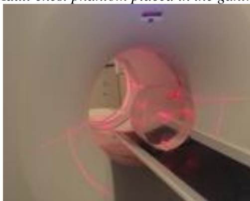
Figure 2: Adult chest phantom placed in the gantry isocenter.
