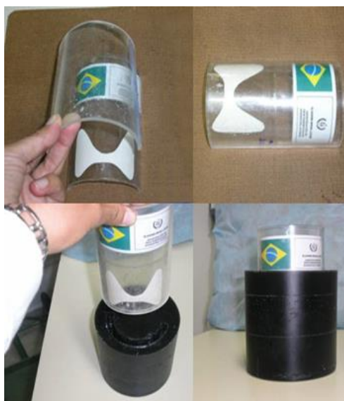
Figure 1: Neck-thyroid phantom produced in the In Vivo Monitoring Laboratory of IRD [6].
