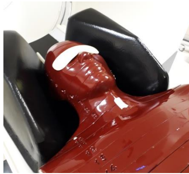
Figure 3: The Alderson phantom with the bismuth shield on the eye spot and a radiochromic film strip on thyroid
