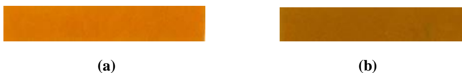
Figure 5: Radiochromic film strips: (a) background and (b) exposed.
