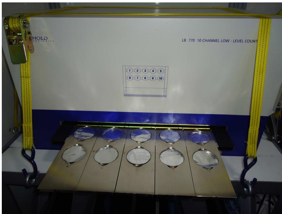
Figure 4: LB770 10 channel low-level conter
