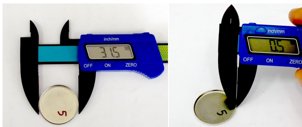
Figure 1: A typical stainless steel sample holder used in LAN-IPEN
